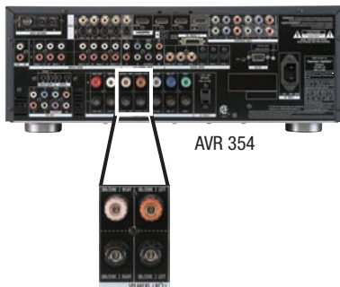
Figure 43 – Surround Back/Zone 2 Speaker Outputs
