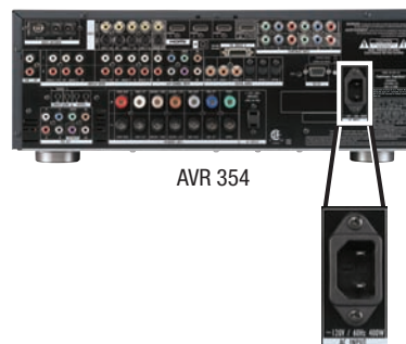
Figure 36 – AC Power Input
